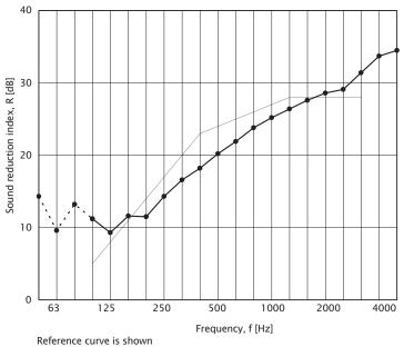
Weighted sound reduction index according to EN ISO 717-1:1996
