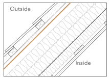
DAFA RooFoil 230 MH Plus used as roof underlay with ventilation between the insulation and the roof underlay.
