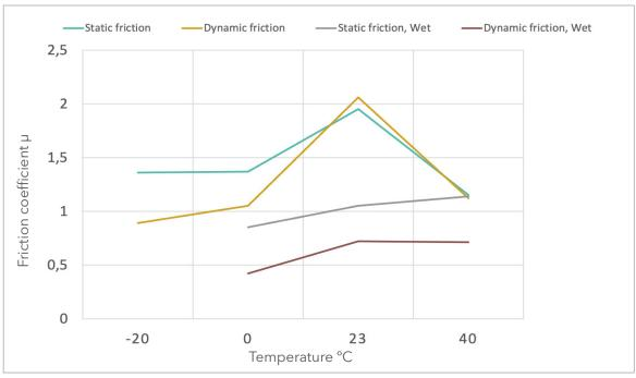
Tested against wind turbine blade coating.
