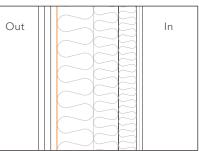
DAFA RooFoil 200 used as a wind barrier with a ventilated cavity behind the rainshield.
